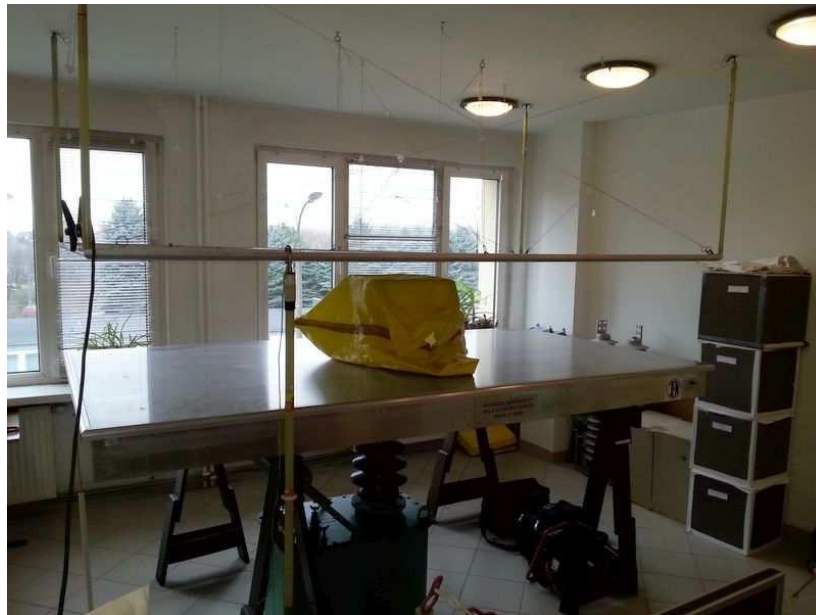
Image 1. Test bench for 50 Hz electric field meters
