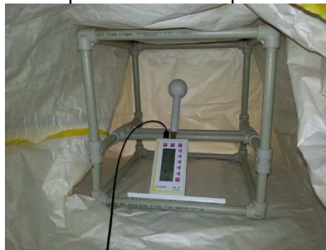
Image 2. View of the test setup with Mascheck ESM-100 meter for testing of electrical field absorption during the test on the tester bench (Test Material 6, cage covered by construction-grade material, interior view)
